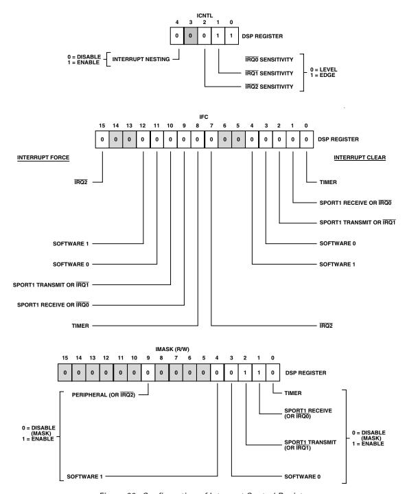
Figure 29. Configuration of Interrupt Control Registers
