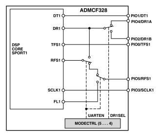
Figure 20. Internal Multiplexing of SPORT1 Pins
