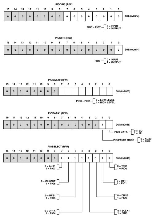
Figure 24. Configuration of PIO Registers
