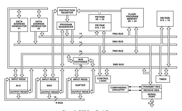
Figure 3. DSP Core Block Diagram
