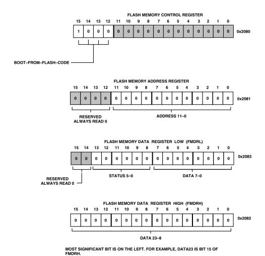
Figure 21. Configuration of Flash Memory Registers
