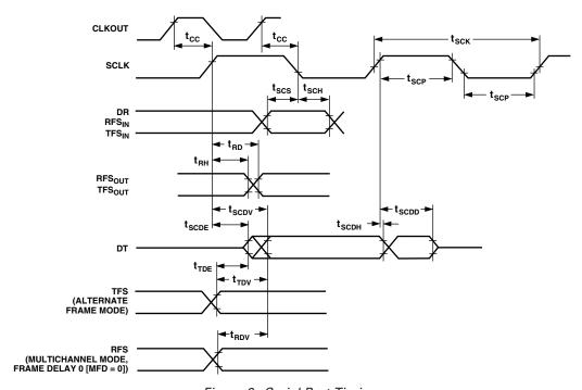
Figure 2. Serial Port Timing
