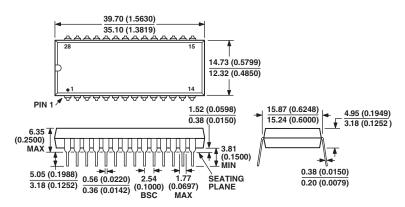
CONTROLLING DIMENSIONS ARE IN MILLIMETERS; INCH DIMENSIONS (IN PARENTHESES) ARE ROUNDED-OFF MILLIMETER EQUIVALENTS FOR REFERENCE ONLY AND ARE NOT APPROPRIATE FOR USE IN DESIGN
