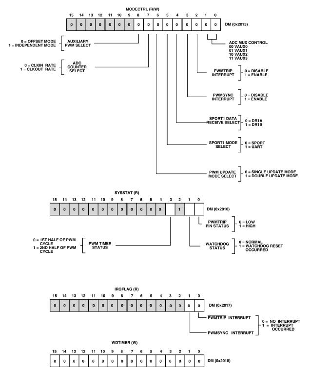
Figure 28. Configuration of Status Registers
