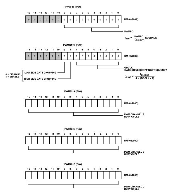
Figure 23. Configuration of Additional PWM Registers
