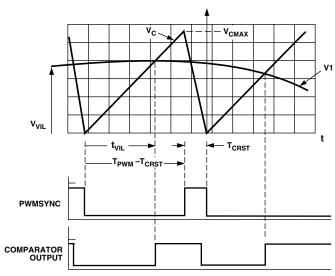
Figure 12. Analog Input Block Operation
