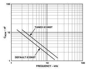
Figure 14. Timing Capacitor Selection
