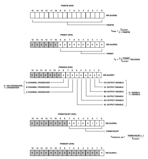
Figure 22. Configuration of PWM Registers
