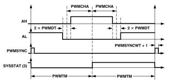
Figure 7. Typical PWM Outputs of Three-Phase Timing Unit in Single Update Mode
