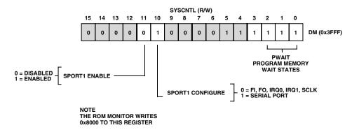
Figure 30. Configuration of Registers
