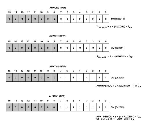
Figure 26. Configuration of AUX Registers
