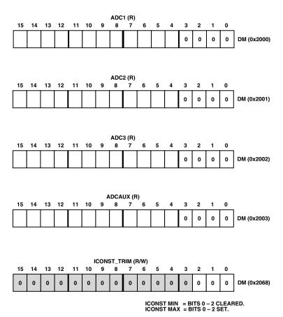
Figure 27. Configuration of Additional AUX Registers
