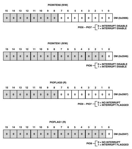
Figure 25. Configuration of Additional PIO Registers
