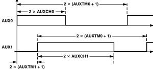
(b) Offset Mode Figure 18. Typical Auxiliary PWM Signals. (All Times in Increments of  $t_{\rm CK}$ )
