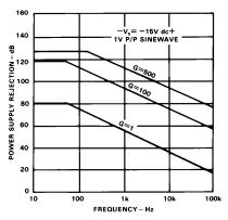
Figure 8. Negative PSRR vs. Frequency
