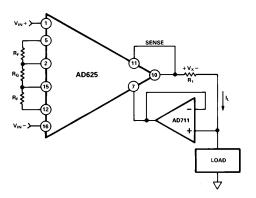
Figure 31. Voltage-to-Current Converter
