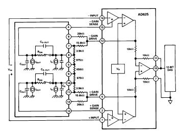
Figure 39. SPGA with Multiplexer Error Sources
