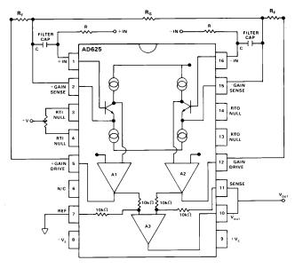
Figure 37. Circuit to Attenuate RF Interference
