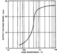
Figure 3. Output Voltage Swing vs. Load Resistance
