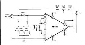
Figure 23. Settling Time Test Circuit
