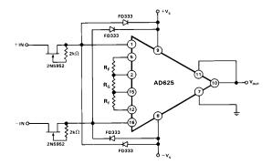
Figure 26c. Input Protection Circuit
