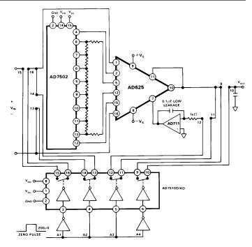
Figure 36. Auto-Zero Circuit
