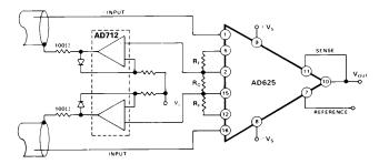
Figure 33. Differential Shield Driver
