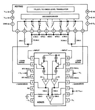
Figure 38. SPGA in a Gain of 16
