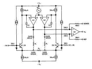
Figure 25. Simplified Circuit of the AD625
