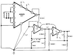
Figure 17. Noise Test Circuit
