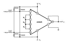
Figure 26a. Input Protection Circuit
