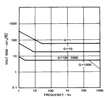
Figure 14. RTI Noise Spectral Density vs. Gain
