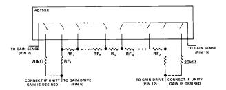
Figure 41. Resistors for a Gain Setting Network
