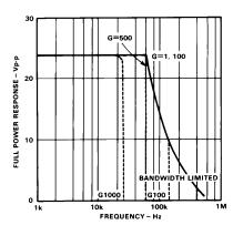
Figure 5. Large Signal Frequency Response
