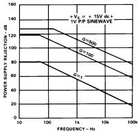
Figure 9. Positive PSRR vs. Frequency
