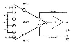
Figure 29. AD625 /Instrumentation Amplifier with Output Current Booster
