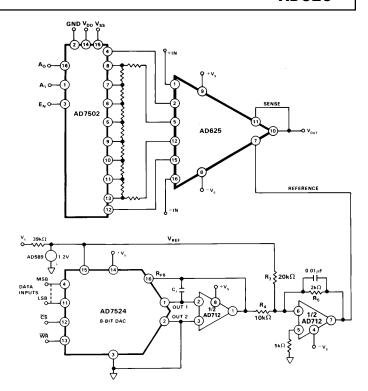
Figure 30. Software Controllable Offset
