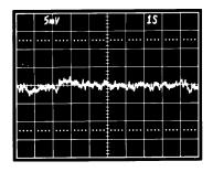
Figure 16. Low Frequency Voltage Noise, G = 1 (System Gain = 1000)
