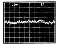
Figure 18. Low Frequency Voltage Noise, G = 1000 (System Gain = 100,000)
