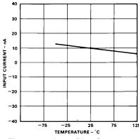
Figure 10. Input Bias Current vs. Temperature
