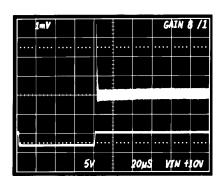
Figure 12. Gain Overrange Recovery
