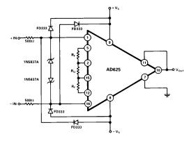
Figure 26b. Input Protection Circuit for G>5
