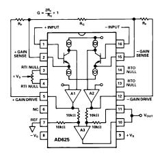
Figure 27. AD625 in Fixed Gain Configuration
