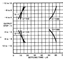
Figure 20. Settling Time to 0.01%
