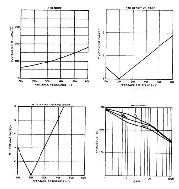
Figure 28. RTO Noise, Offset, Drift and Bandwidth vs. Feedback Resistance Normalized to 20  $k\Omega$
