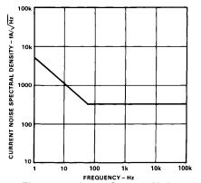
Figure 15. Input Current Noise
