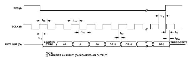
Figure 10. External Clocking (Slave) Mode Output Register Read
