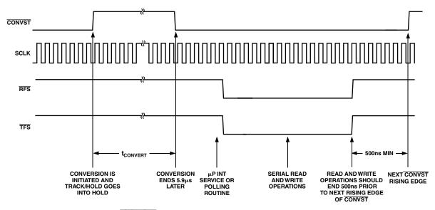
Figure 6. CONVST Used as Status Signal in External Clocking Mode
