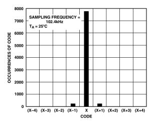
Figure 19. Histogram of 8192 Conversions with Write During Conversion
