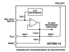
Figure 2. AD7890-10 Analog Input Structure
