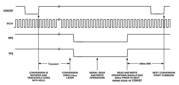
Figure 5. External Clocking (Slave) Mode Timing Sequence for Optimum Performance
