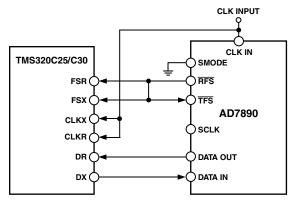
Figure 16. AD7890 to TMS320C25/30 Interface
