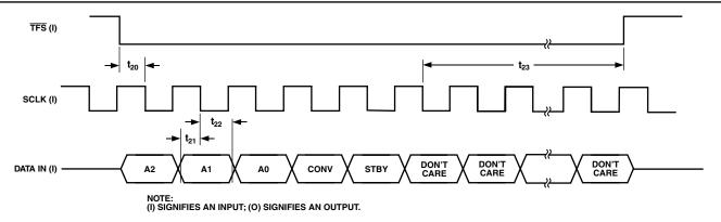
Figure 11. External Clocking (Slave) Mode Control Register Write
