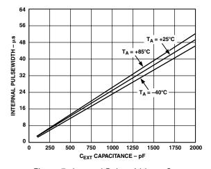
Figure 7. Internal Pulsewidth vs.  $C_{EXT}$
