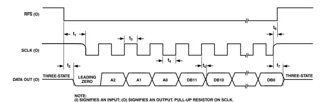
Figure 8. Self-Clocking (Master) Mode Output Register Read
