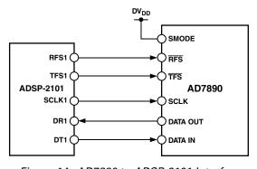
Figure 14. AD7890 to ADSP-2101 Interface
