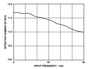
Figure 21. Effective Number of Bits vs. Frequency
