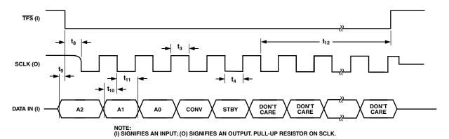
Figure 9. Self-Clocking (Master) Mode Control Register Write
