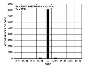
Figure 17. Histogram of 8192 Conversions of a DC Input
