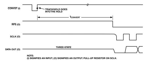
Figure 4. Self-Clocking (Master) Mode Conversion Sequence
