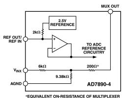
Figure 3. AD7890-4 Analog Input Structure
