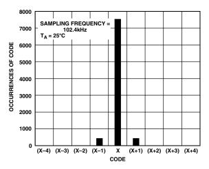
Figure 18. Histogram of 8192 Conversions with Read During Conversion
