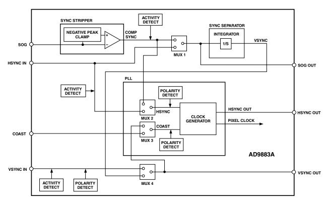
Figure 12. Sync Processing Block Diagram
