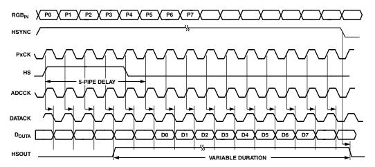
Figure 8. 4:4:4 Mode (For RGB and YUV)
