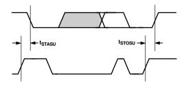
Figure 10. Serial Port Read/Write Timing
