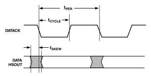
Figure 7. Output Timing
