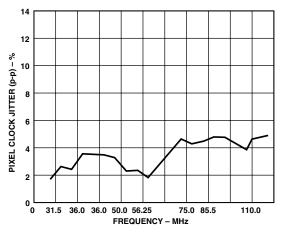
Figure 5. Pixel Clock Jitter vs. Frequency
