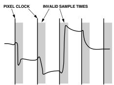
Figure 4. Pixel Sampling Times
