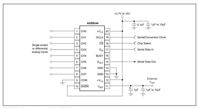
FIGURE 1. Basic Operation of the ADS8344.
