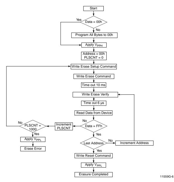
Figure 1. Flasherase Electrical Erase Algorithm
