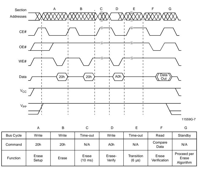
Figure 2. AC Waveforms For Erase Operations
