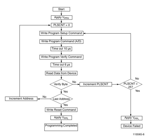
Figure 3. Flashrite Programming Algorithm
