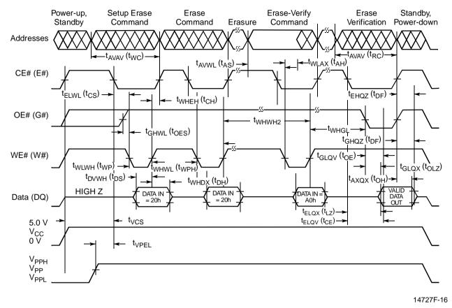
Figure 8. AC Waveforms for Erase Operations
