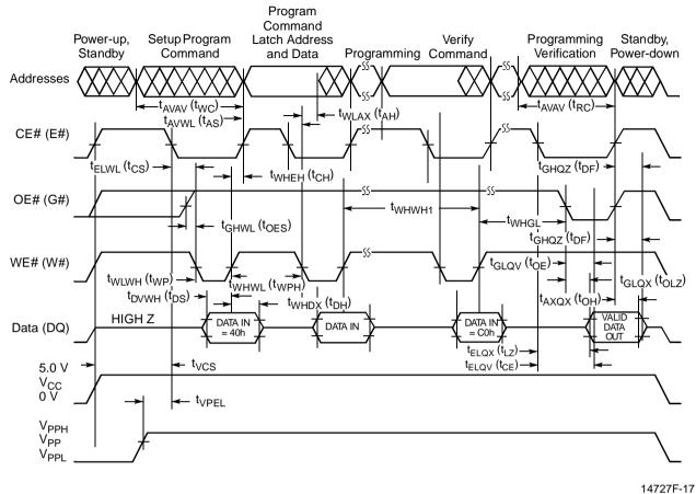
Figure 9. AC Waveforms for Programming
