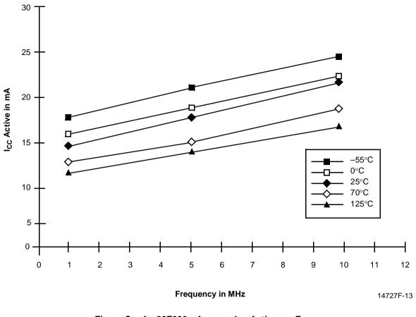
Figure 5. Am28F020—Average I<sub>CC</sub> Active vs. Frequency VCC = 5.5 V, Addressing Pattern = Minmax Data Pattern = Checkerboard
