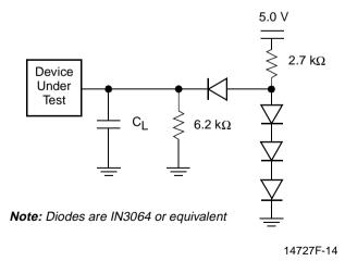
Figure 6. Test Setup
