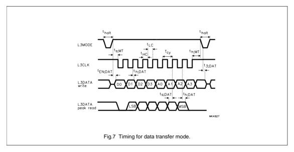
All transfers are bytewise, i.e. they are based on groups of 8 bits. Data will be stored in the TDA1546T after the eighth bit of a byte has been received.
