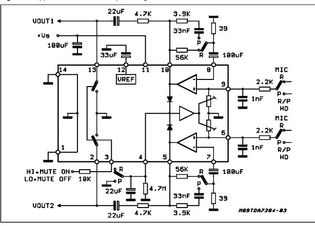
Figure 22: Application Circuit with Output Muting
