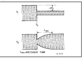
The recovery time (Trec) is defined as the time between the instant To and the instant in which the output signal returns to the nominal level.
