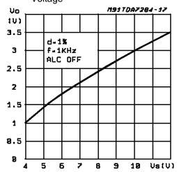
Figure 8: Output Voltage vs. Input Voltage
