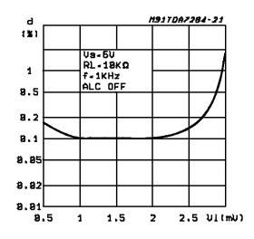
Figure 11: Distortion vs. Input Voltage
