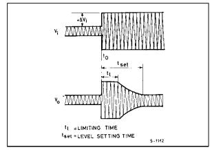
Usually such an increase drives the op-amp into saturation and the time for which it remains in this condition is called the limiting time(T1).
