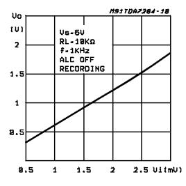
Figure 9: Output Voltage vs. Input Voltage
