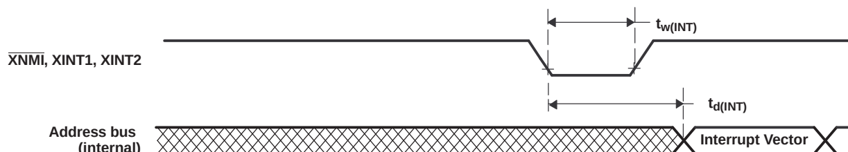
Figure 6-17. External Interrupt Timing
