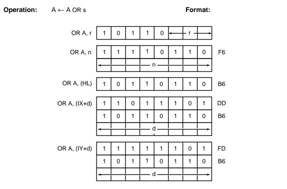
**Description:** The s operand is logically inclusive ORed with the value in the Accumulator A, the result is stored in A, and the flags are set as described below. "s" can be any of a register r, an "immediate" value n in the instruction itself, a memory location selected by the contents of the HL register pair, or a memory location selected by the sum of the contents of an index register IX or IY and a signed 8-bit displacement d. In
