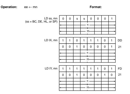
**Description:** The 16-bit "immediate" value mn in the instruction is loaded into register ee. The flags are not affected. "ee" can be any of the register pairs BC, DE, or HL, the Stack Pointer SP, or an index register IX or IY. "n" is loaded into the less-significant half
