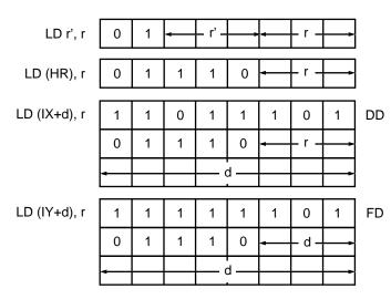
**Description:** The value of the source register r is loaded into the m operand. The flags are not affected. "m" can be any of a destination register r' a memory location selected by the contents of the HL register pair, or a memory location selected by the sum of the contents of an index register IX or IY and a signed 8-bit displacement d. r selects a source register, and in the
