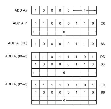
**Description:** The s operand is added to the value in the Accumulator (A), the result is stored in A, and the flags are set as described below. "s" can be any of a register r, an "immediate" value n in the instruction itself, a memory location selected by the contents of the HL register pair, or a memory location selected by the sum of the contents of an index register IX or IY and a signed 8-bit displacement d. In the register form, r selects a source register as follows:
