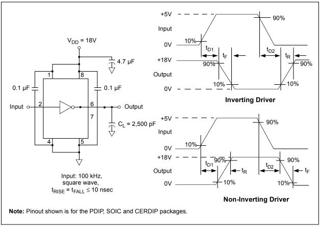
FIGURE 4-1: Switching Time Test Circuits.
