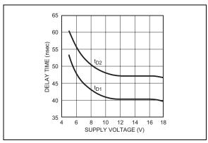
FIGURE 2-8: Supply Voltage.
