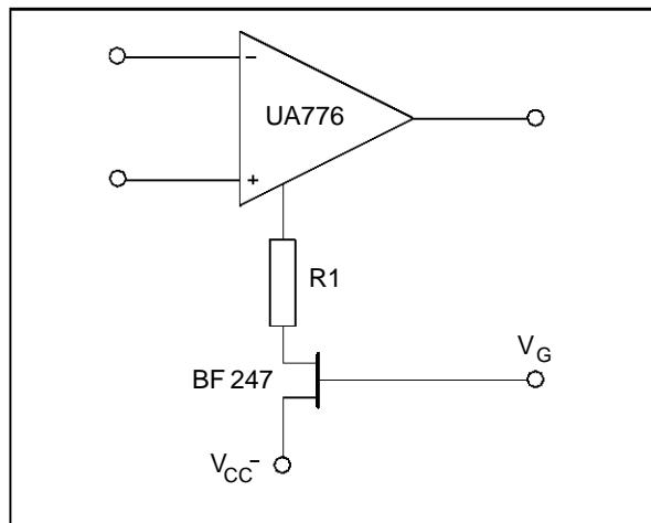
**OFFSET VOLTAGE NULL CIRCUIT**
