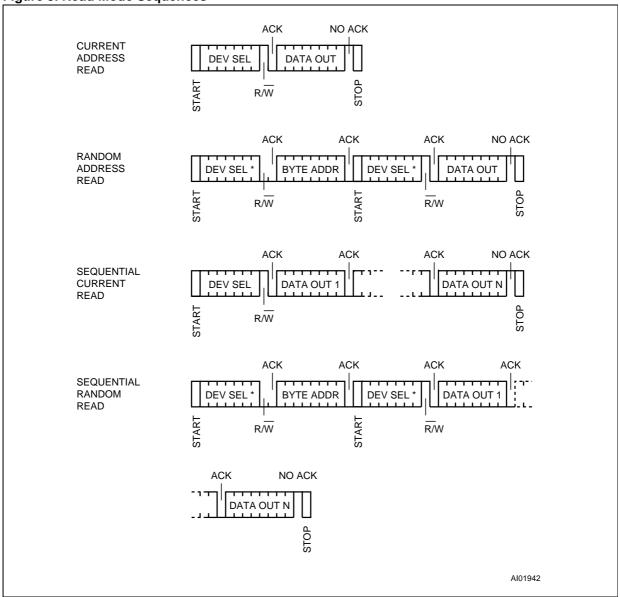
Note: 1. The seven most significant bits of the Device Select Code of a Random Read (in the 1<sup>st</sup> and 3<sup>rd</sup> bytes) must be identical.
