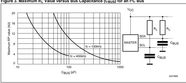
Figure 3. Maximum R<sub>L</sub> Value versus Bus Capacitance (C<sub>BUS</sub>) for an I<sup>2</sup>C Bus
