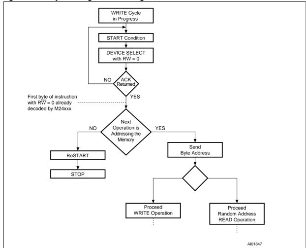
Figure 7. Write Cycle Polling Flowchart using ACK
