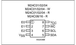
Note: 1. Pin 1 is Not Connected for 4 Kbit devices
