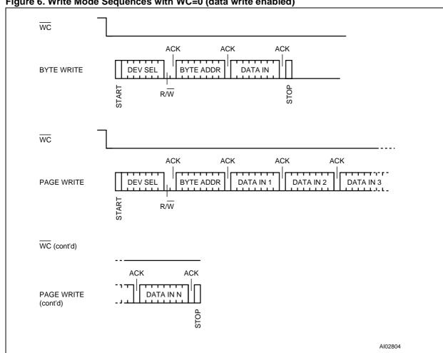
Figure 6. Write Mode Sequences with WC=0 (data write enabled)
