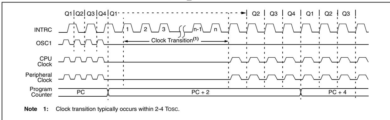
**FIGURE 3-4: TRANSITION TIMING FROM RC\_RUN MODE TO PRI\_RUN MODE**
