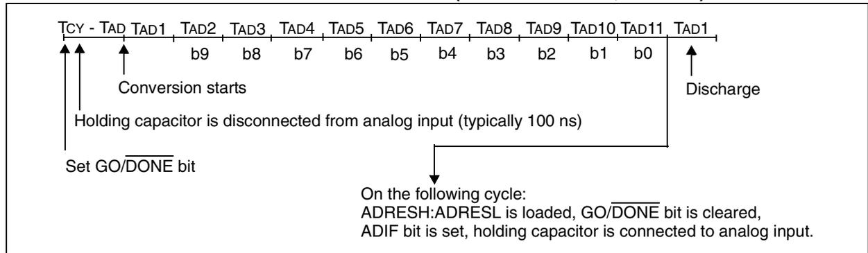
**FIGURE 16-5: A/D CONVERSION TAD CYCLES (ACQT<2:0> = 010, TACQ = 4 TAD)**
