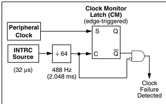
Clock failure is tested for on the falling edge of the sample clock. If a sample clock falling edge occurs while CM is still set, a clock failure has been detected (Figure 18-4). This causes the following:
