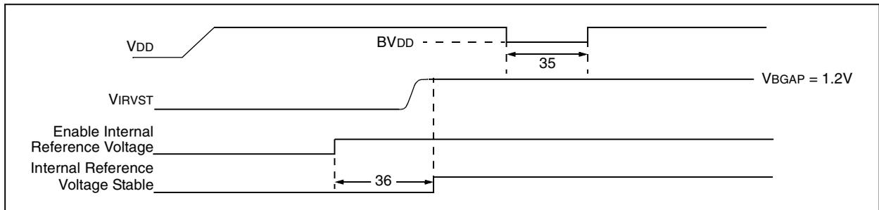
**TABLE 21-10: RESET, WATCHDOG TIMER, OSCILLATOR START-UP TIMER, POWER-UP TIMER AND BROWN-OUT RESET REQUIREMENTS**
