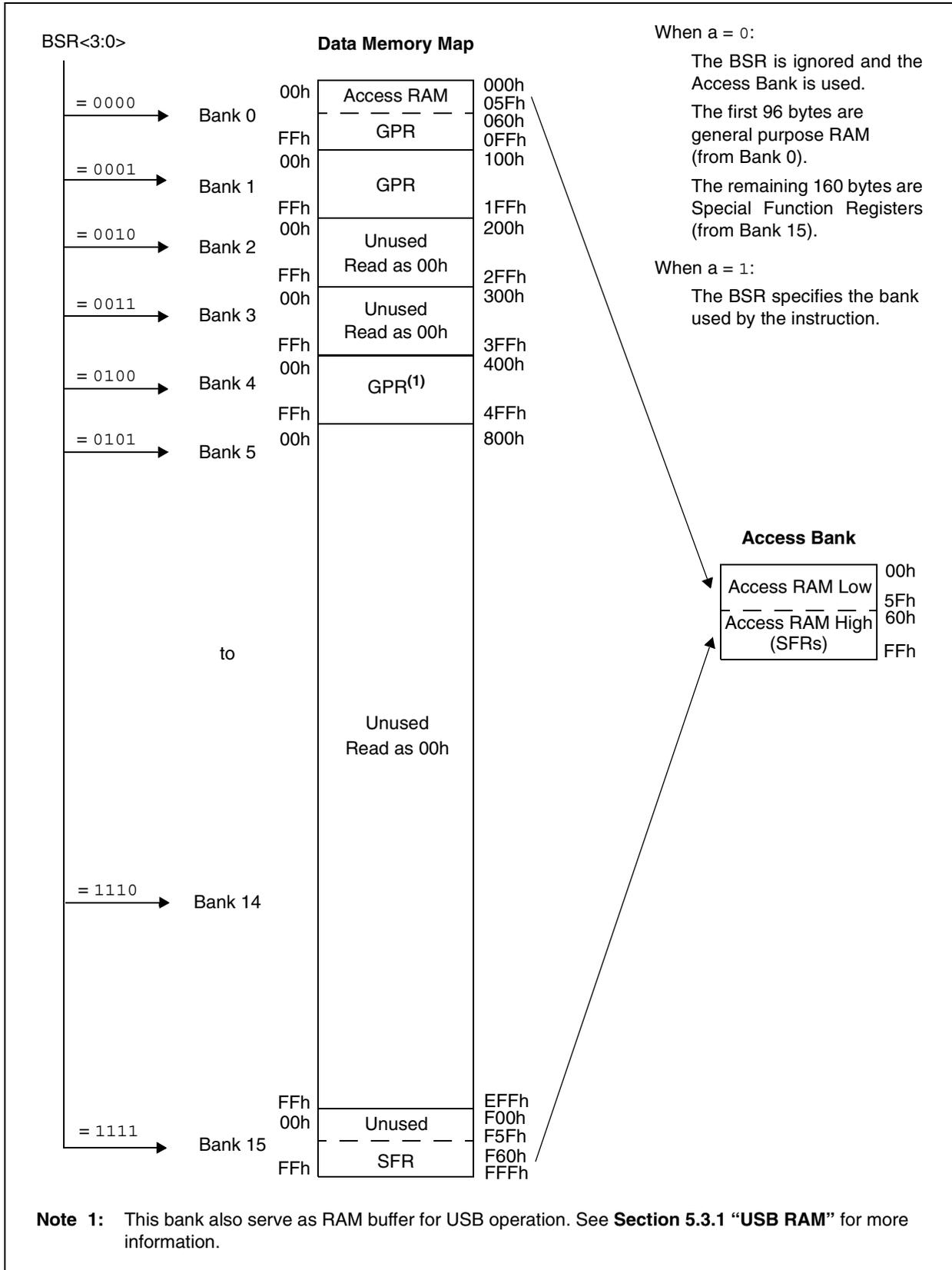
**FIGURE 5-6: USE OF THE BANK SELECT REGISTER (DIRECT ADDRESSING)**
