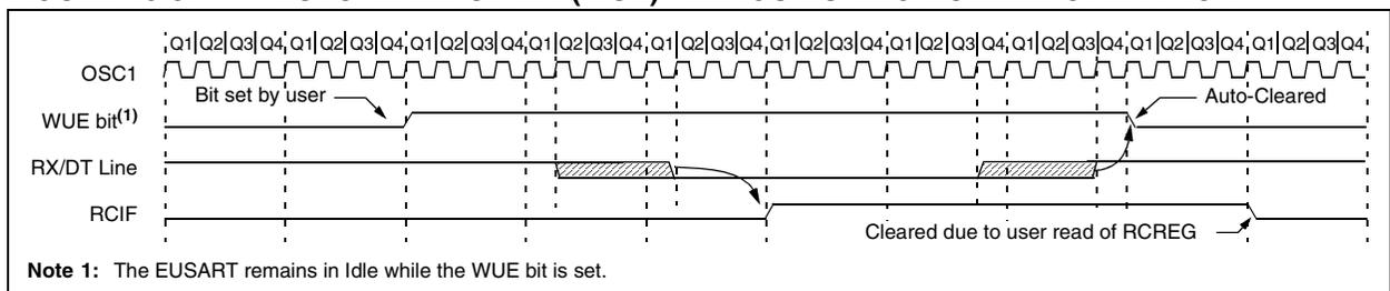
**FIGURE 15-9: AUTO-WAKE-UP BIT (WUE) TIMINGS DURING SLEEP**
