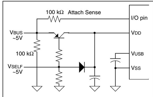
**Note:** Users should keep in mind the limits for devices drawing power from the USB. According to USB Specification 2.0, this cannot exceed 100 mA per low-power device or 500 mA per high-power device.
