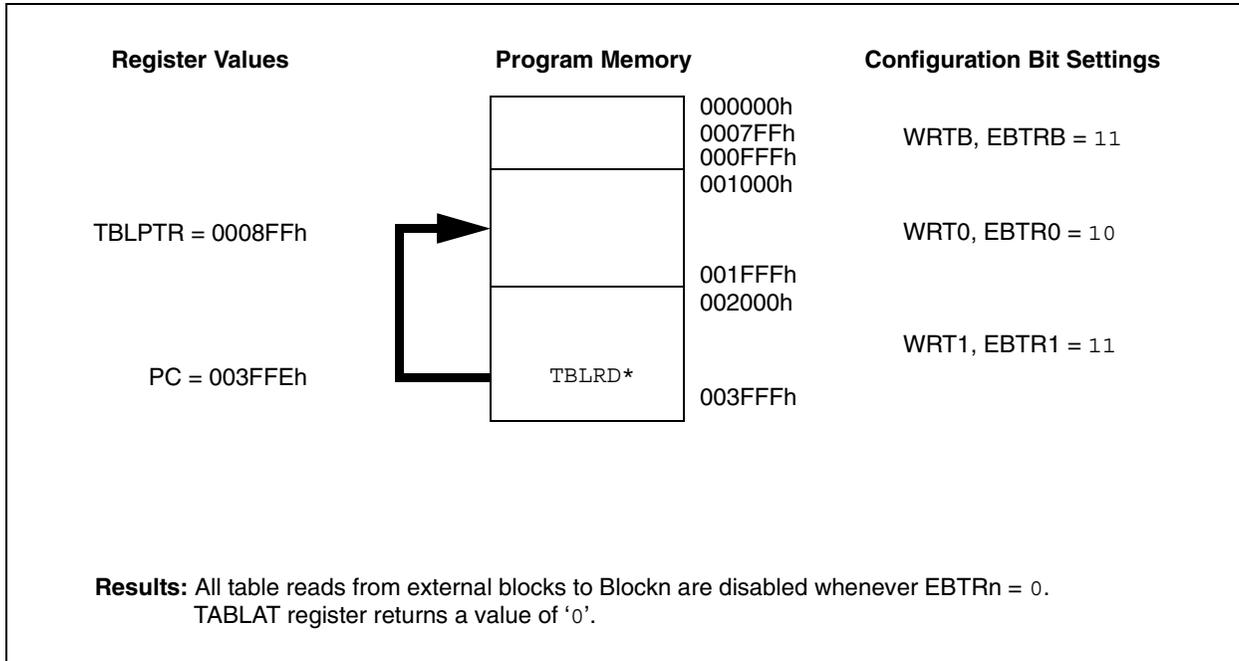
**FIGURE 18-8: EXTERNAL BLOCK TABLE READ (EBTRn) ALLOWED**
