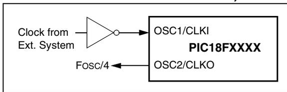
The ECIO and ECPIO Oscillator modes function like the EC and ECPLL modes, except that the OSC2 pin becomes an additional general purpose I/O pin. The I/O pin becomes bit 6 of PORTA (RA6). Figure 2-5 shows the pin connections for the ECIO Oscillator mode.
