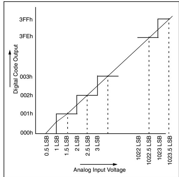
**FIGURE 16-3: ANALOG INPUT MODEL**
