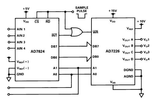
Figure 20. 4-Channel Fast Infinite Sample-and-Hold
