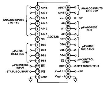
Figure 4. AD7828 Operational Diagram
