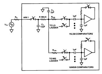
Figure 8. AD7824/AD7828 Equivalent Input Circuit
