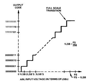
Figure 11. Ideal Input/Output Transfer Characteristic for Unipolar 0 V to +5 V Operation
