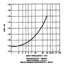
Signal-Noise Ratio vs. Input Frequency
