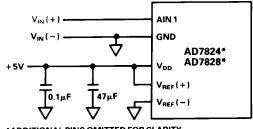
\*ADDITIONAL PINS OMITTED FOR CLARITY, ONLY CHANNEL 1 SHOWN
