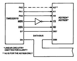
Figure 18. AD7824/AD7828-TMS32010 Interface
