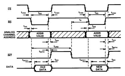
Figure 15. Mode 1 Timing Diagram
