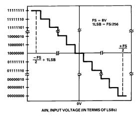
Figure 13. Ideal Input/Output Transfer Characteristic for ±4 V Operation
