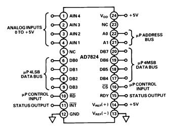
Figure 3. AD7824 Operational Diagram
