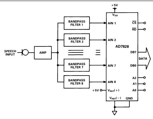
Figure 19. Speech Analysis Using Real-Time Filtering
