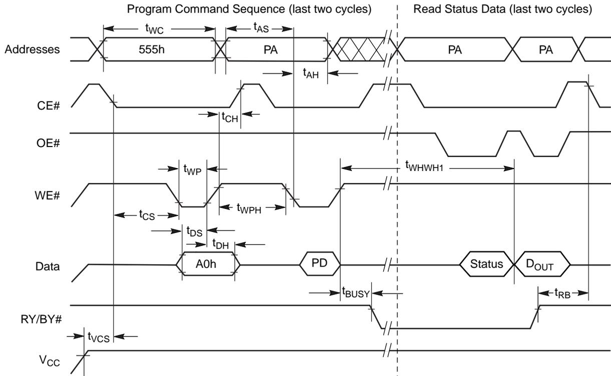
Note: PA = program address, PD = program data, D<sub>OUT</sub> is the true data at the program address.
