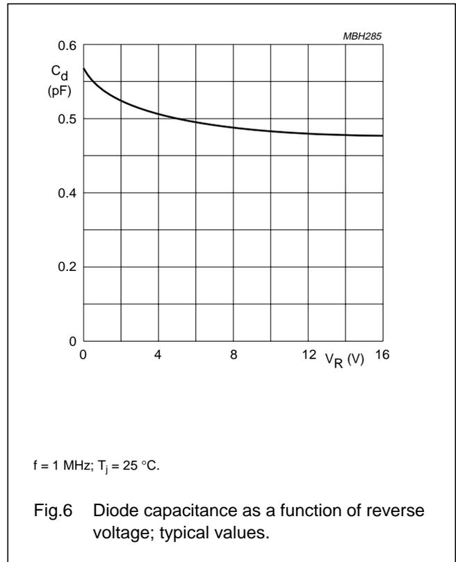
High-speed switching diode
