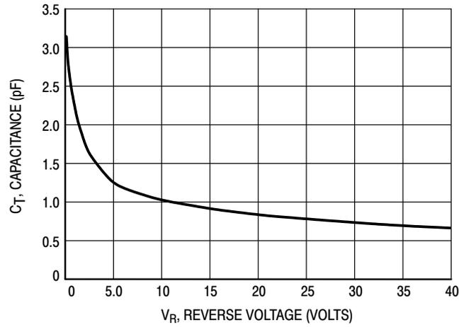
Figure 3. Typical Capacitance
