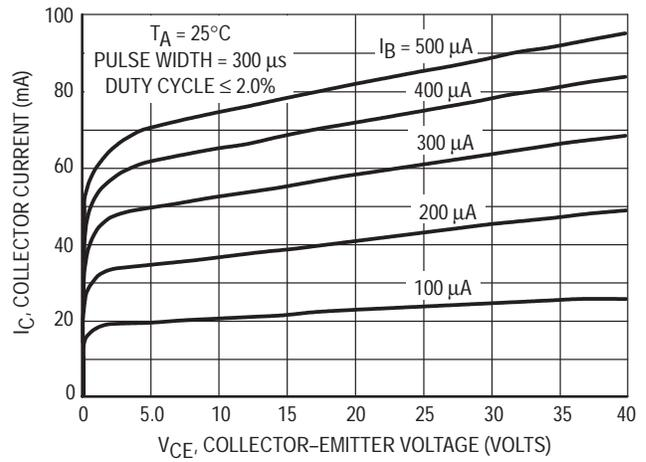
Figure 8. Collector Characteristics
