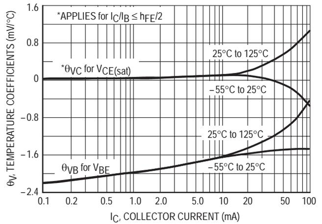
Figure 10. Temperature Coefficients
