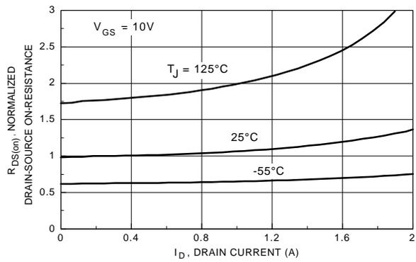
Figure 4. On-Resistance Variation with Drain Current and Temperature.
