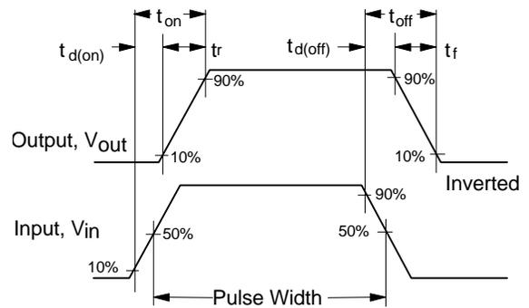
**Figure 12. Switching Waveforms.**
