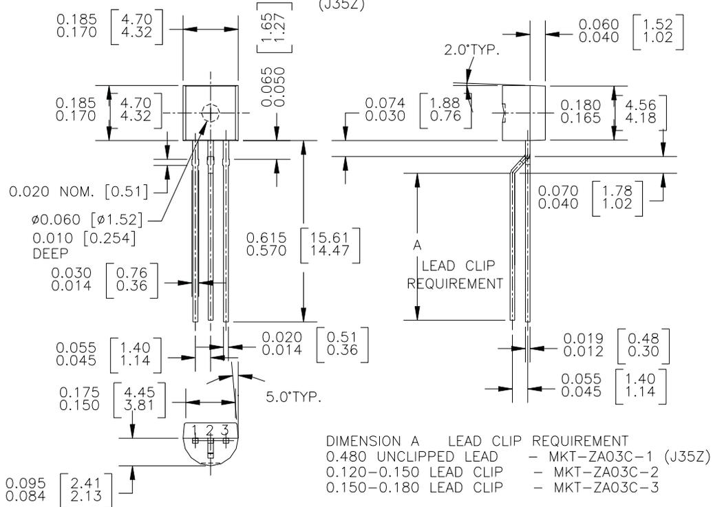
**Note:** All package 97 or 98 transistors are leadformed to this configuration prior to bulk shipment. Order L34Z option if in-line leads are preferred on package 97 or 98.
