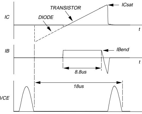
Fig.1. Switching times waveforms.
