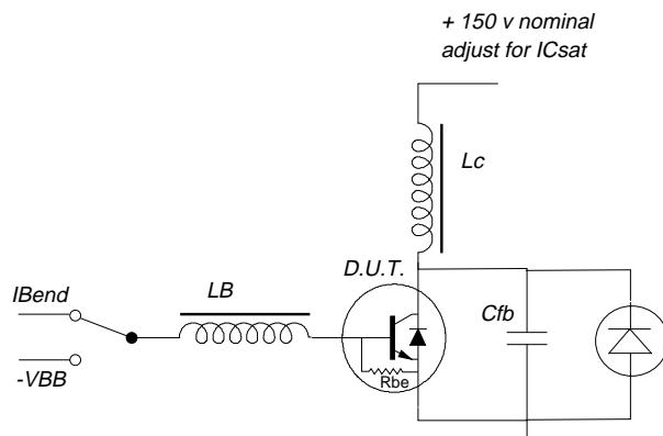
Fig.4. Switching times test circuit.
