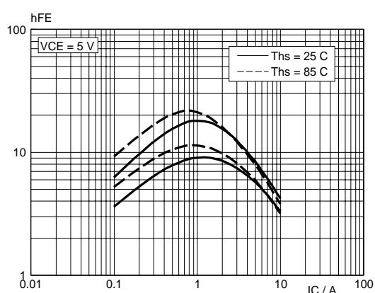
Fig.6. High and low DC current gain.  $h_{FE} = f (I_C)$
