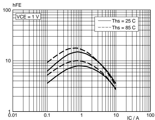
Fig.5. High and low DC current gain.  $h_{FE} = f (I_C)$
