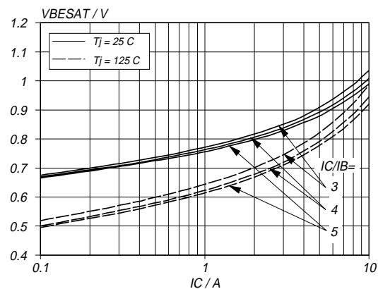
Fig.7. Typical base-emitter saturation voltage.
