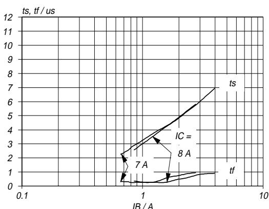
Fig.12. Typical collector storage and fall time.
