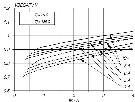
Fig.9. Typical base-emitter saturation voltage.
