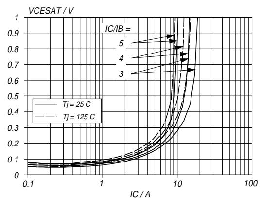
Fig.8. Typical collector-emitter saturation voltage.
