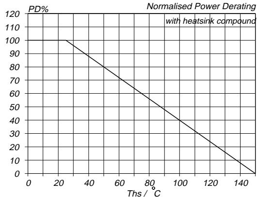
Fig.13. Normalised power dissipation.
