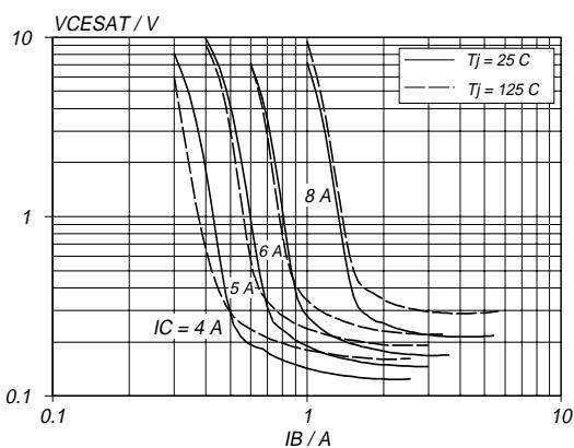
Fig.10. Typical collector-emitter saturation voltage.
