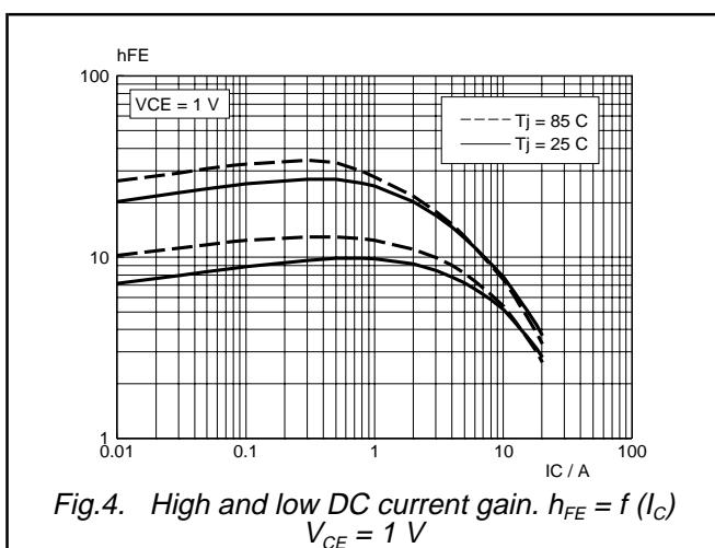
Fig.4. High and low DC current gain.
