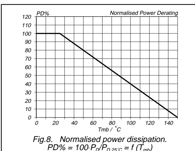
Fig.8. Normalised power dissipation.
