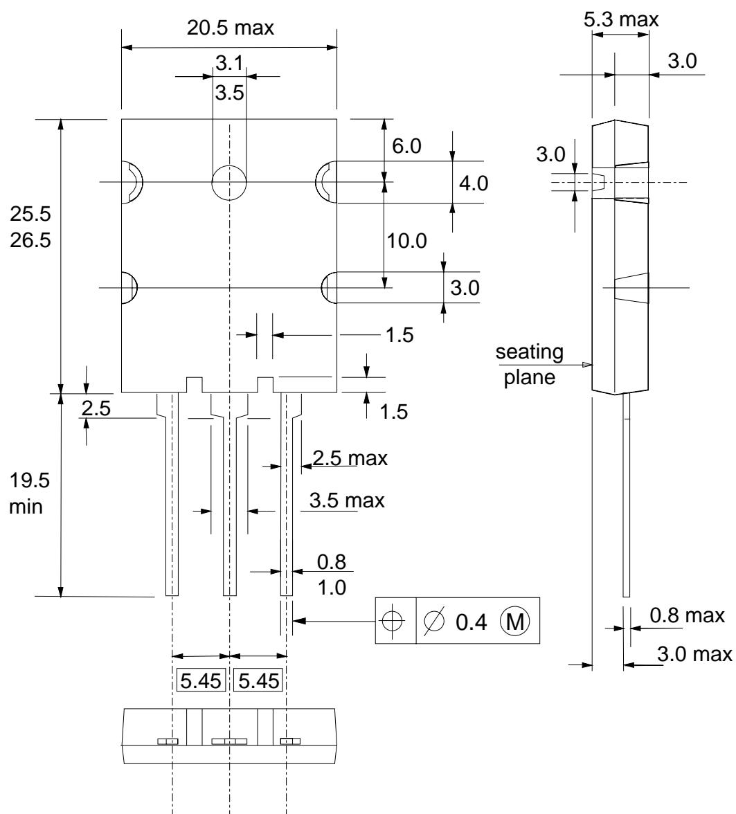
Fig.12. SOT430; pin 2 connected to mounting base.
