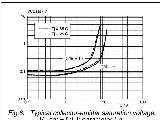
Fig.6. Typical collector-emitter saturation voltage.
