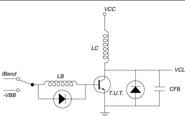
Fig.10. Test Circuit RBSOA.  $V_{CC} = 150$  V;
