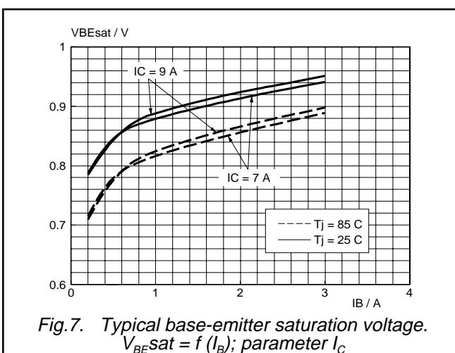
Fig.7. Typical base-emitter saturation voltage.
