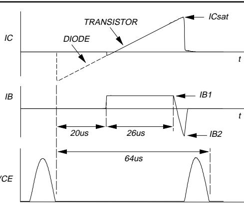
Fig.3. Switching times waveforms (16 kHz).
