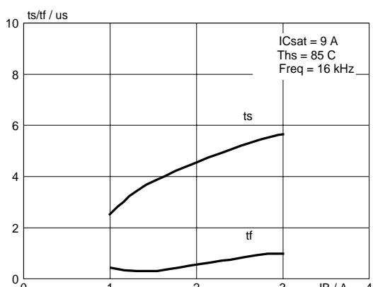
Fig.9. Typical collector storage and fall time.
