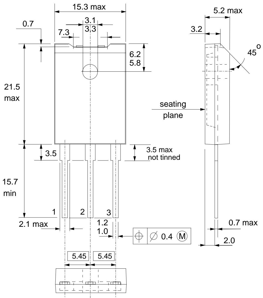
Fig.13. SOT199; The seating plane is electrically isolated from all terminals.
