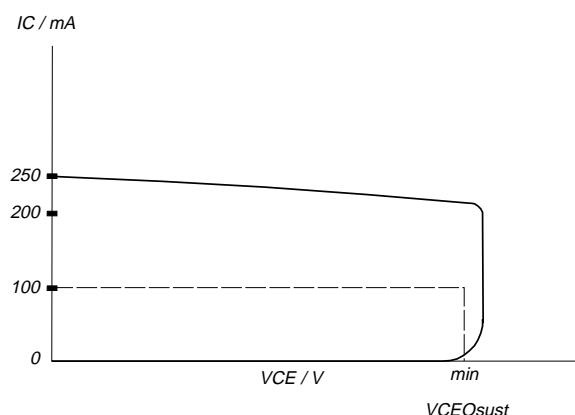
Fig.2. Oscilloscope display for  $V_{CEO_sust}$ .
