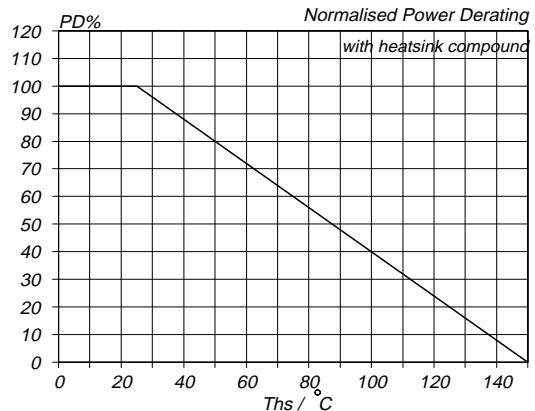
Fig.10. Normalised power dissipation.
