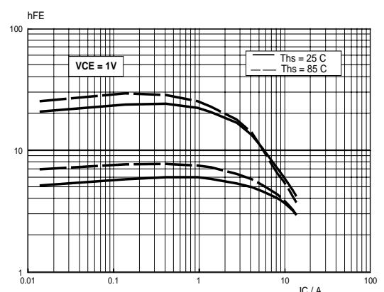
Fig.6. High and low DC current gain.
