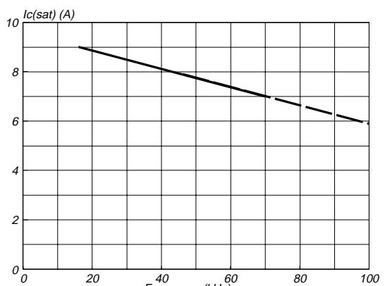
Fig.12.  $I_{C,sat}$  during normal running vs. frequency of operation for optimum performance
