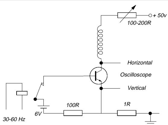
Fig.1. Test circuit for  $V_{CEO_sust}$ .
