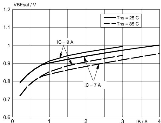
Fig.8. Typical base-emitter saturation voltage.
