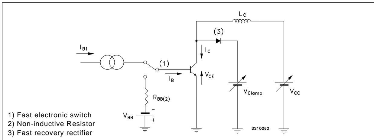
**Figure 2:** Resistive Load Switching Test Circuit.
