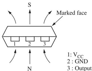
Applying direction of magnetic flux
