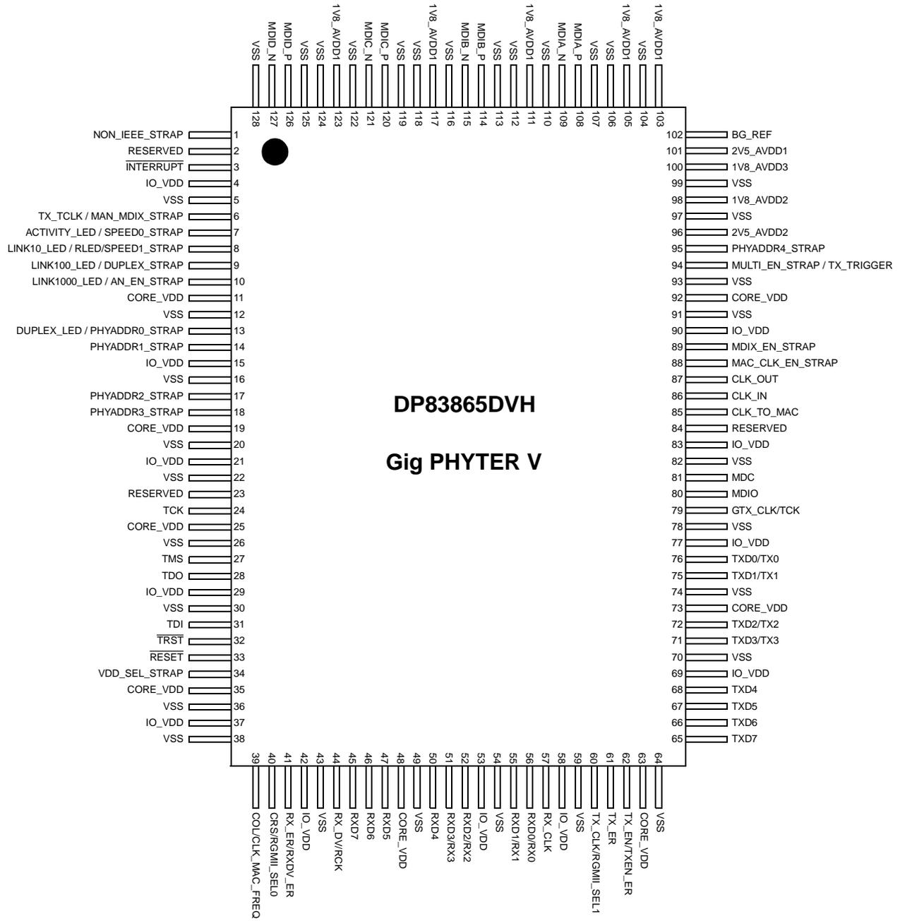
Figure 1. DP83865 Pinout
