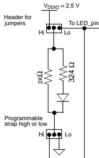
Figure 20. LED/strapping option examples.
