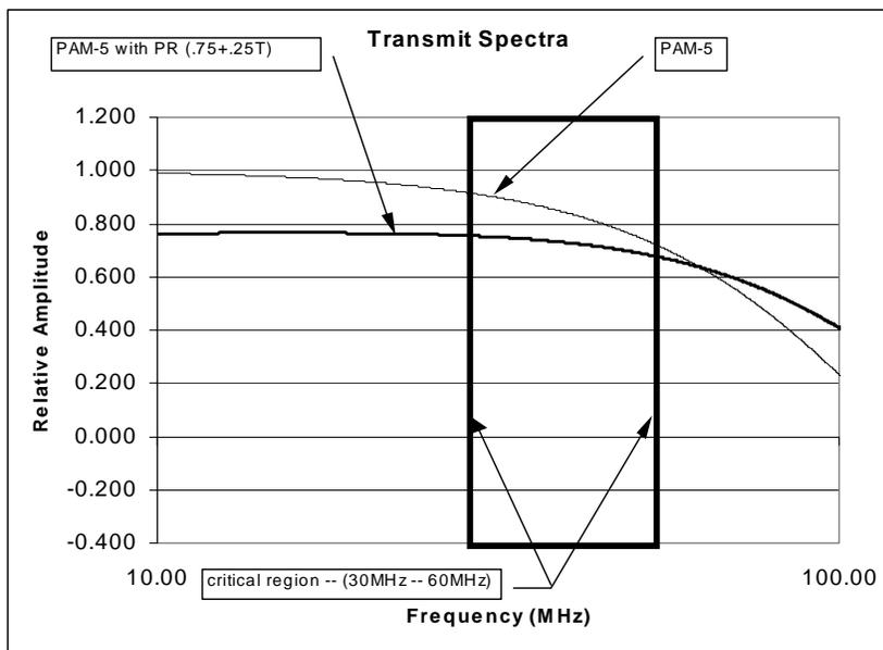
Figure 4. Effect on Spectrum of PR-shaped PAM-5 coding
