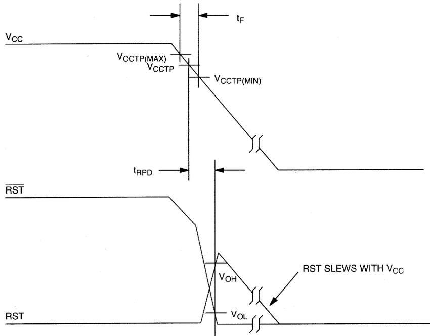
**TIMING DIAGRAM: POWER UP Figure 8**
