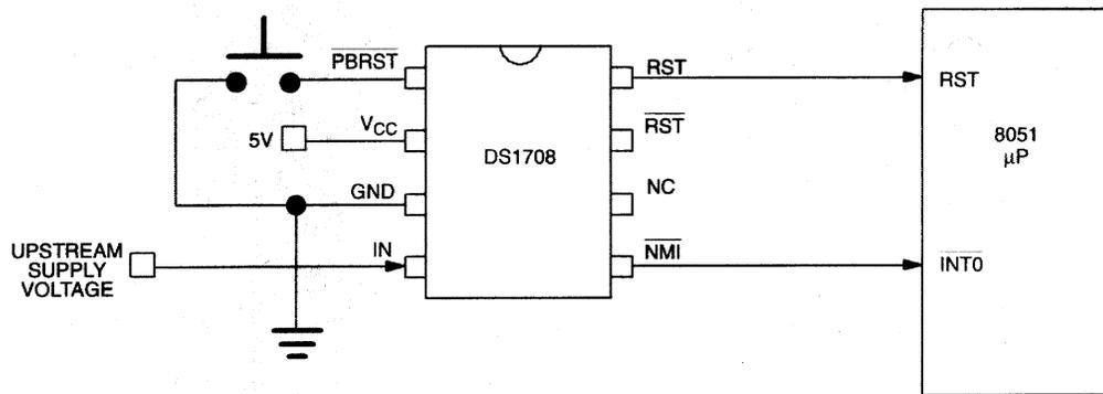
**PUSHBUTTON RESET CONTROLLED BY NMI Figure 3**
