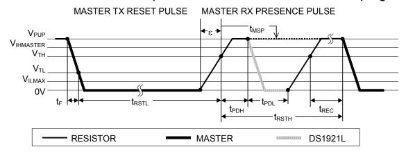
After the bus master has released the line it goes into receive mode (RX). Now, the 1-Wire bus is pulled to  $V_{PUP}$  via the pull-up resistor or, in case of a DS2480B driver, by active circuitry. When the threshold  $V_{TH}$  is crossed, the DS1921L waits for  $t_{PDH}$  and then transmits a Presence Pulse by pulling the line low for  $t_{PDL}$ . To detect a presence pulse, the master must test the logical state of the 1-Wire line at  $t_{MSP}$ .
