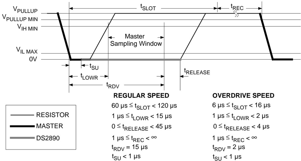
\*The optimal sampling point for the master is as close as possible to the end time of the  $t_{RDV}$  period without exceeding  $t_{RDV}$ . For the case of a Read-one time slot, this maximizes the amount of time for the pull-up resistor to recover the line to a high level. For a Read-zero time slot it ensures that a read will occur before the fastest 1-Wire device(s) release the line ( $t_{RELEASE} = 0$ ).
