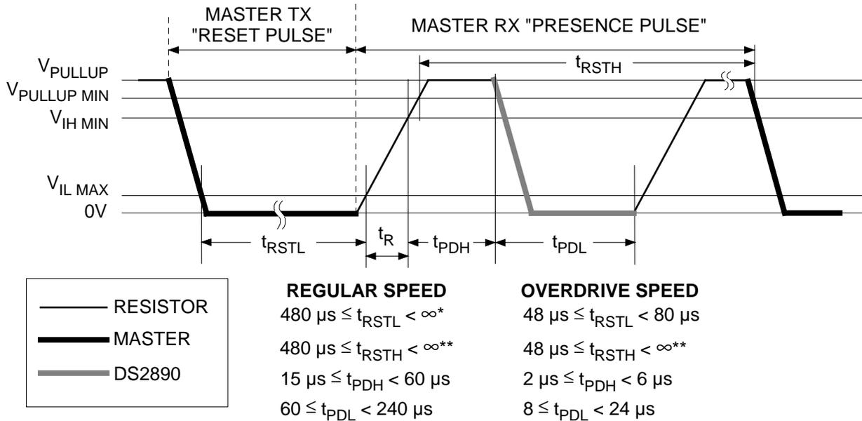
\* In order not to mask interrupt signaling by other devices on the 1-Wire bus and to prevent a power-on reset of the parasite powered circuit,  $t_{RSTL} + t_R$  should always be less than 960  $\mu s$ .
