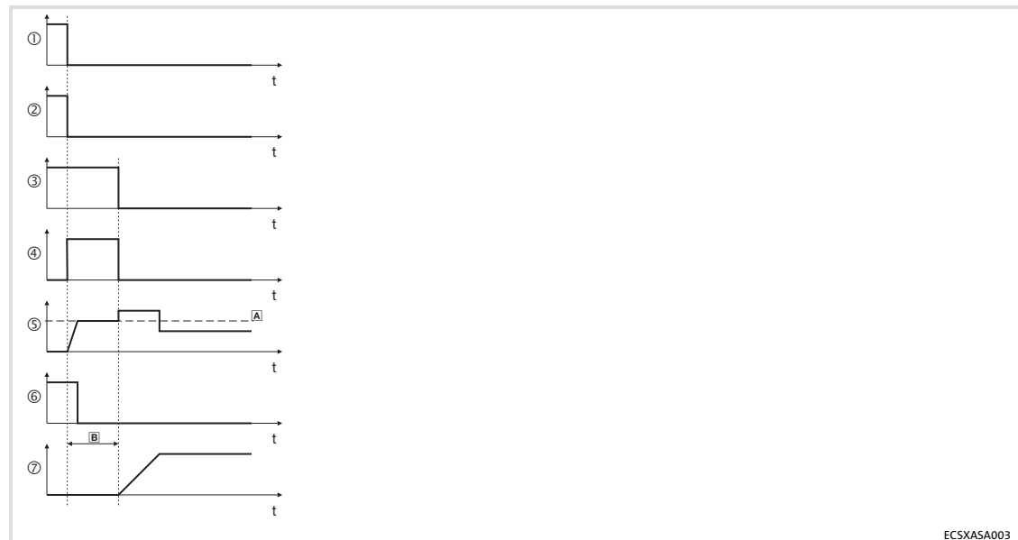
Fig.11-37 Signal characteristic - opening of holding brake
