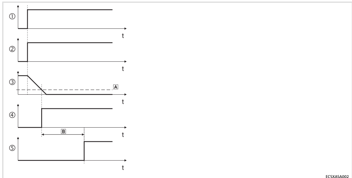
Fig.11-31 Signal characteristic - closing of holding brake
