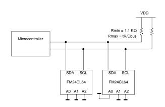
Figure 2. Typical System Configuration
