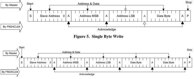
Figure 6. Multiple Byte Write
