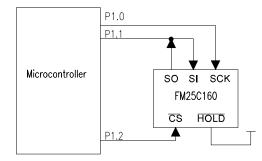
Figure 3. System Configuration without SPI port
