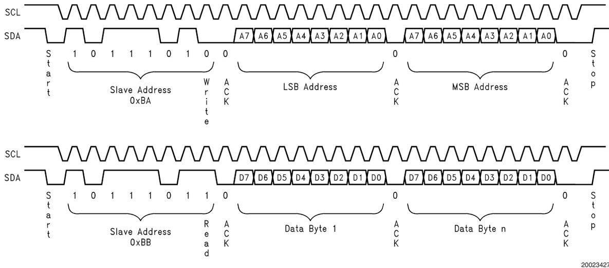
**FIGURE 20. I<sup>2</sup>C Compatible Read Sequence**
