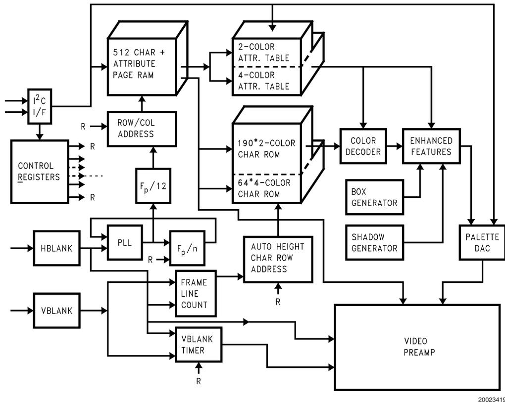
FIGURE 12. Block Diagram of the OSD Generator
