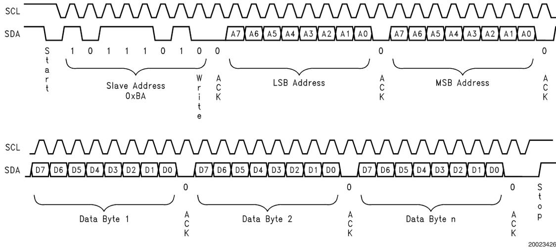
**FIGURE 19. I<sup>2</sup>C Compatible Write Sequence**
