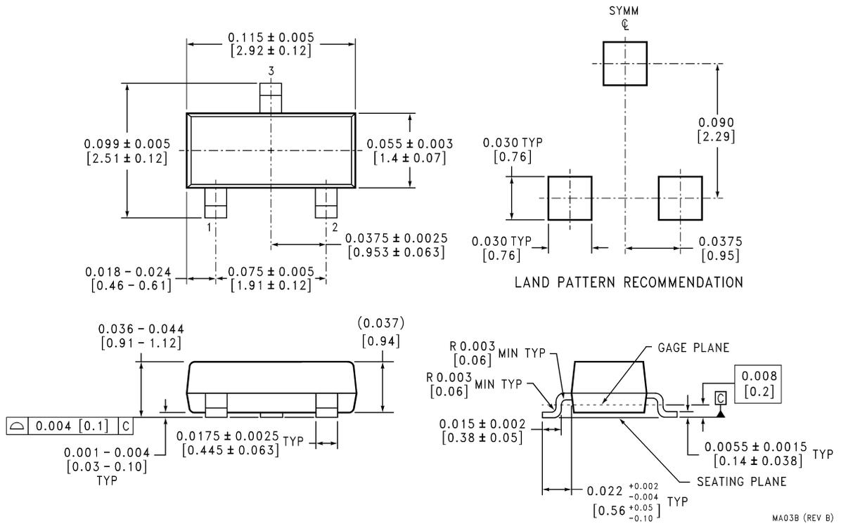
**SOT-23 Molded Small Outline Transistor Package (M3)**
