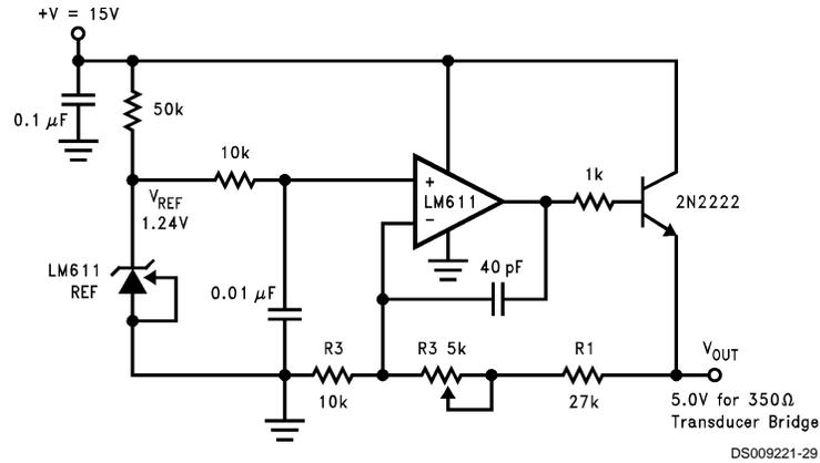
$V_{OUT} = (R1/R2 + 1) V_{REF}$ .
