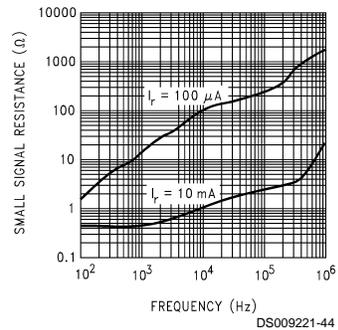
**Typical Performance Characteristics (Reference)**  $T_J = 25^\circ\text{C}$ , FEEDBACK pin shorted to  $V^- = 0\text{V}$ , unless otherwise noted (Continued)
