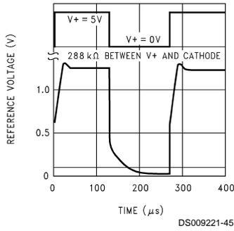
**Reference Voltage with Feedback Voltage Step**
