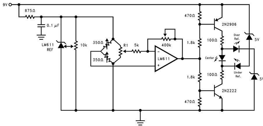
**FIGURE 16. Nulling Bridge Detection System.** Adjust sensitivity via 400 kΩ pot.
