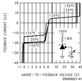
**Feedback Current vs Feedback-to-Anode Voltage**
