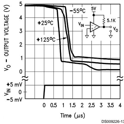
Comparator Response Times — Non-Inverting Input, Positive Transition
