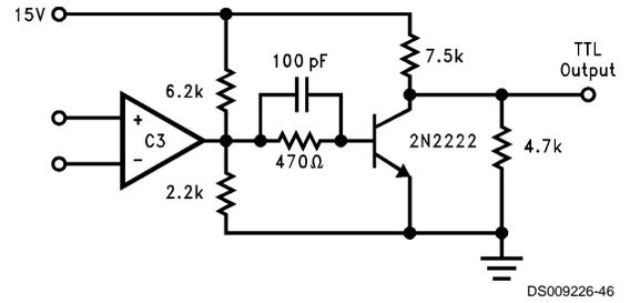
FIGURE 17. Wide-Input Range Comparator with TTL Output
