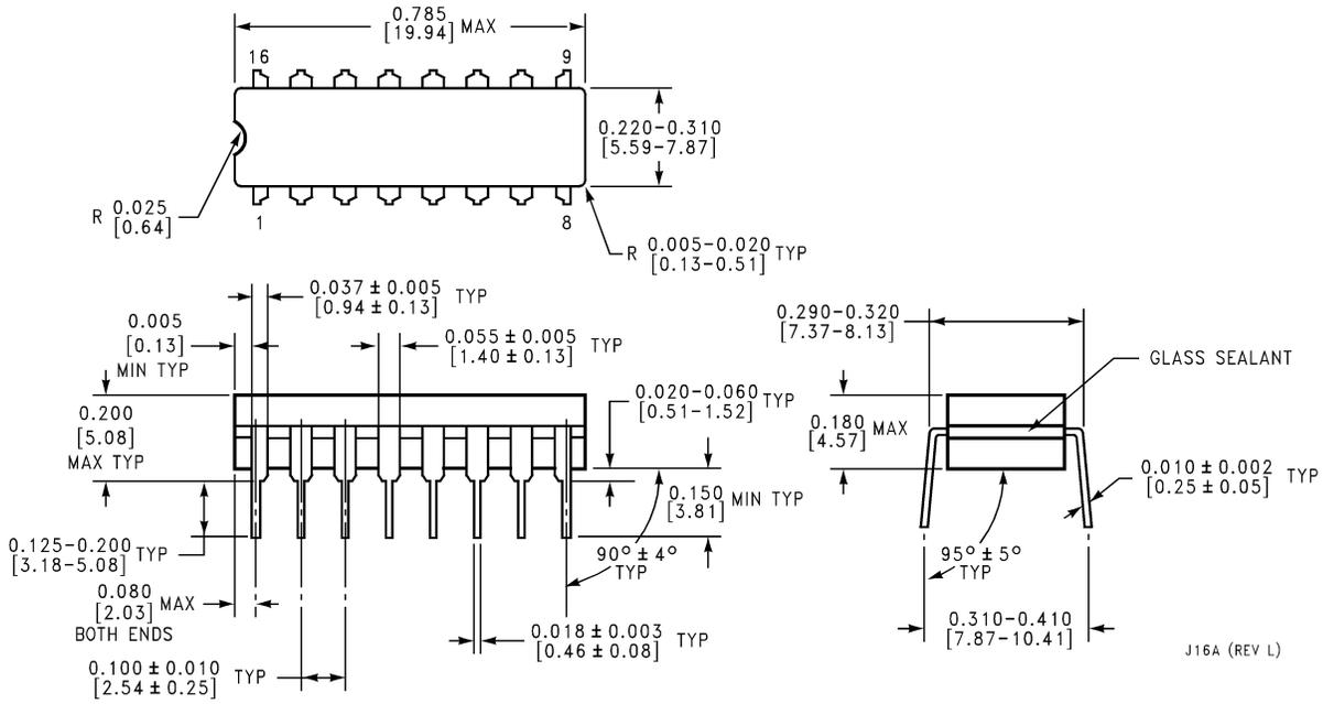
**16-Lead Ceramic Dual-In-Line Package (J)**
