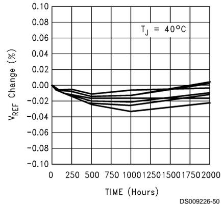
**Accelerated Reference Voltage Drift vs Time**
