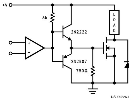
FIGURE 12. High Current, High Voltage Switch
