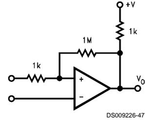
FIGURE 18. Comparator with Hysteresis ( $\Delta V_H = +V(1k/1M)$ )
