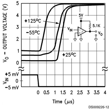
Comparator Response Times — Inverting Input, Negative Transition
