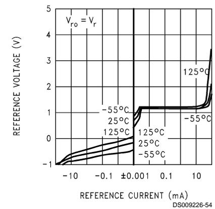
**Typical Performance Characteristics (Reference)**  $T_J = 25^\circ\text{C}$ , FEEDBACK pin shorted to  $V^- = 0\text{V}$ , unless otherwise noted (Continued)
