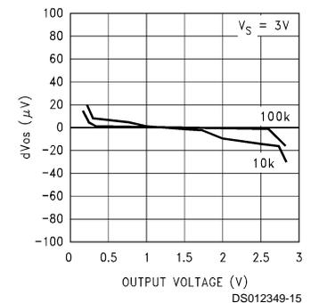
**Typical Performance Characteristics**  $T_A = 25^\circ\text{C}$ ,  $R_L = 10\text{ k}\Omega$  unless otherwise specified (Continued)
