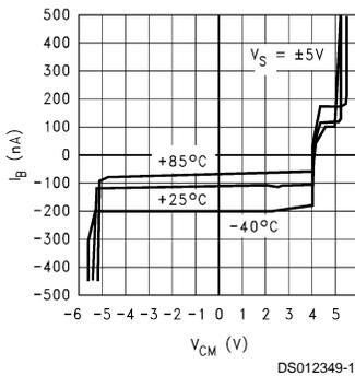
**Input Bias Current vs Supply Voltage**
