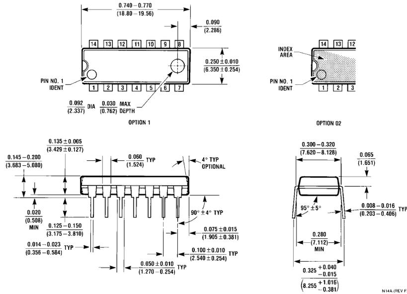
**14-Lead (0.300" Wide) Molded Dual-In-Line Package**
