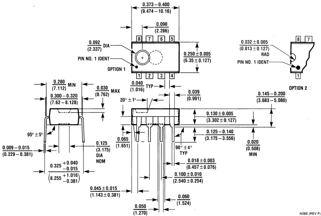
**8-Pin Molded Dual-In-Line Package**
