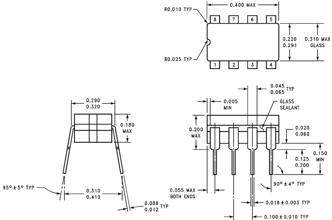
**8-Pin Ceramic Dual-In-Line Package**
