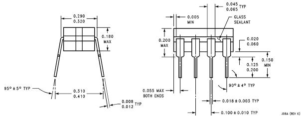
8-Pin Ceramic Dual-In-Line Package Order Number LMC6062AMJ/883 **NS Package Number J08A**
