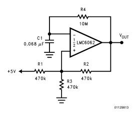
FIGURE 9. 1 Hz Square Wave Oscillator
