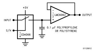
FIGURE 8. Low-Leakage Sample and Hold
