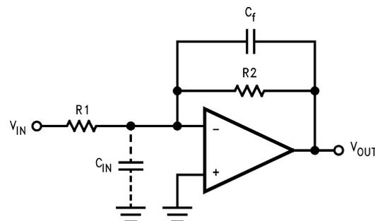
FIGURE 1. Cancelling the Effect of Input Capacitance
