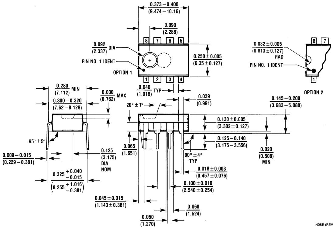
**8-Lead (0.300" Wide) Molded Dual-In-Line Package**
