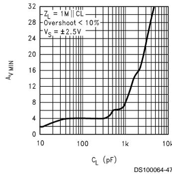
FIGURE 4. Minimum Operating Gain vs Capacitive Load
