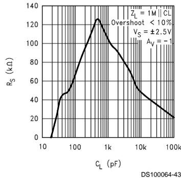
FIGURE 5. Isolating Resistor Value vs Capacitive Load
