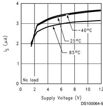
**Total Supply Current vs Supply Voltage (Positive Input Overdrive)**
