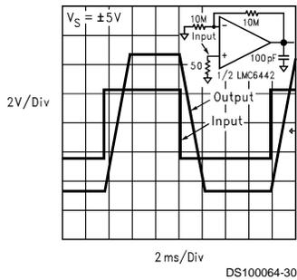
**Small Signal Step Response (AV = -1) (CL=1MΩ || 100 pF, 200 pF)**
