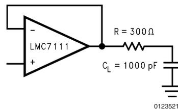
FIGURE 2. Resistive Isolation of a 330 pF Capacitive Load
