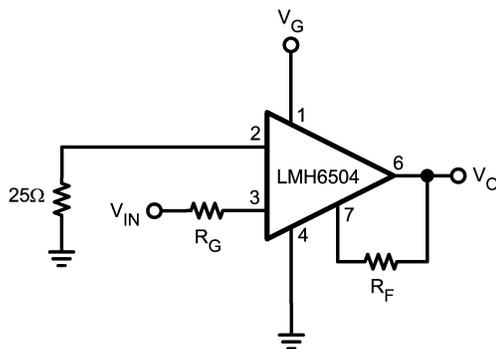
FIGURE 4. Inverting Amplifier
