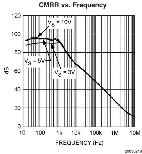
**Typical Performance Characteristics** At  $T_J = 25^\circ\text{C}$ ,  $V^+ = +2.5$ ,  $V^- = -2.5$ ,  $R_F = 330\Omega$  for  $A_V = +2$ ,  $R_F = 1\text{k}\Omega$  for  $A_V = -1$ . Unless otherwise specified. (Continued)
