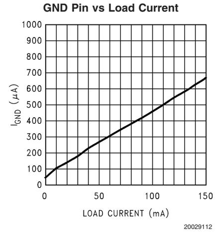
**Typical Performance Characteristics** Unless otherwise specified:  $C_{IN} = 1\mu F$ ,  $C_{OUT} = 2.2\mu F$ ,  $V_{IN} = V_{OUT(NOM)} + 1$ ,  $T_A = 25^\circ C$ , ON/OFF pin is tied to  $V_{IN}$ . (Continued)
