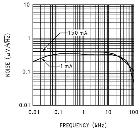
**Typical Performance Characteristics** Unless otherwise specified:  $C_{IN} = 1\mu F$ ,  $C_{OUT} = 2.2\mu F$ ,  $V_{IN} = V_{OUT(NOM)} + 1$ ,  $T_A = 25^\circ C$ , ON/OFF pin is tied to  $V_{IN}$ . (Continued)
