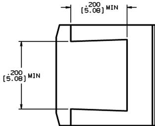
**TO263 5-Lead, Molded, Surface Mount Package (TO263-5)**
