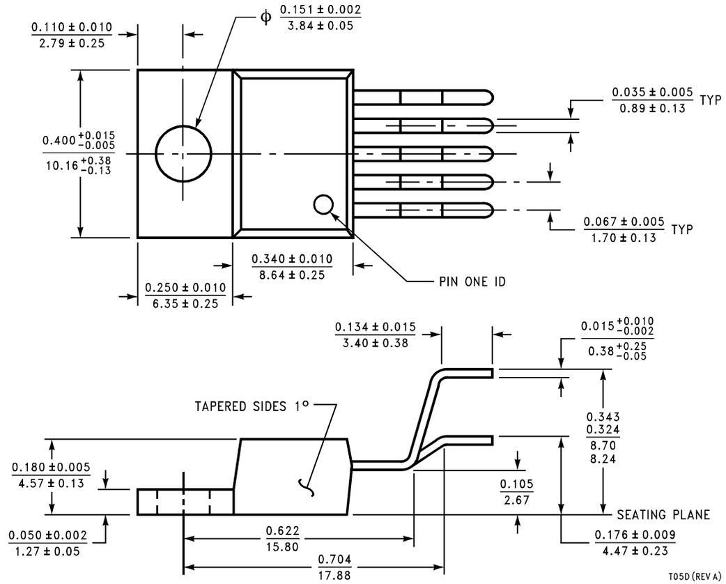
**TO220 5-lead, Molded, Stagger Bend Package (TO220-5)
