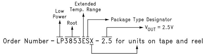
Package Type Designator is "T" for TO220 package, and "S" for TO263 package.
