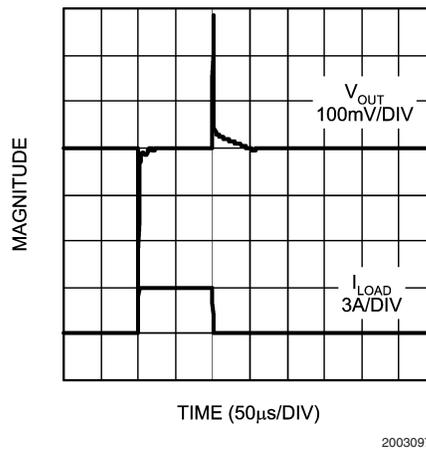
**Typical Performance Characteristics** Unless otherwise specified:  $T_J = 25^\circ\text{C}$ ,  $C_{OUT} = 10\mu\text{F}$ ,  $C_{IN} = 10\mu\text{F}$ , S/D pin is tied to  $V_{IN}$ ,  $V_{OUT} = 2.5\text{V}$ ,  $V_{IN} = V_{O(NOM)} + 1\text{V}$ ,  $I_L = 10\text{mA}$ . (Continued)
