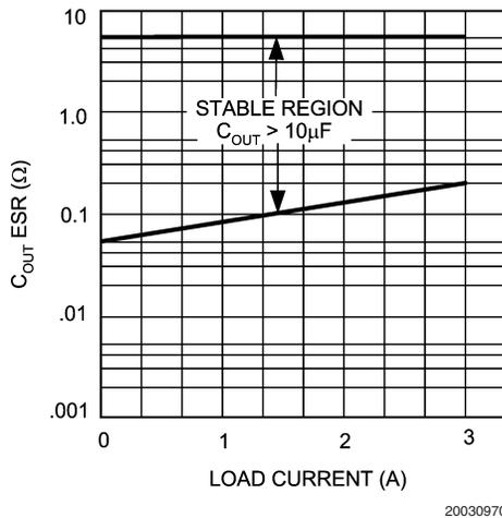
**FIGURE 1. ESR Curve for C<sub>OUT</sub> (with 10 $\mu$ F Tantalum Input Capacitor)**
