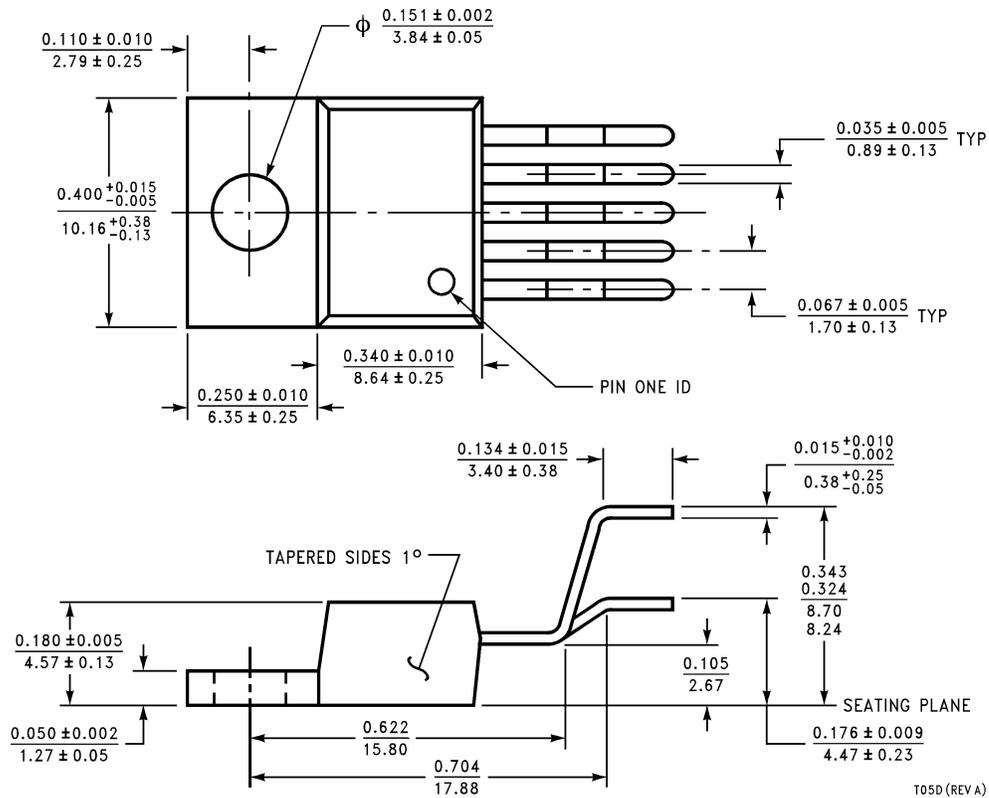
**TO220 5-lead, Molded, Stagger Bend Package (TO220-5)
