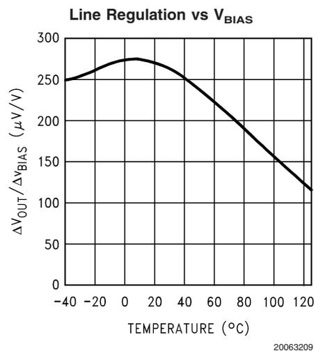
**Typical Performance Characteristics** Unless otherwise specified:  $T_A = 25^\circ\text{C}$ ,  $C_{OUT} = 4.7\mu\text{F}$ ,  $C_{in} = 4.7\mu\text{F}$ ,  $\overline{\text{S/D}}$  pin is tied to  $V_{BIAS}$ ,  $V_{IN} = 2.2\text{V}$ ,  $V_{OUT} = 1.8\text{V}$ . (Continued)
