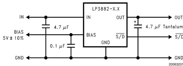
At least 4.7 μF of input and output capacitance is required for stability.
