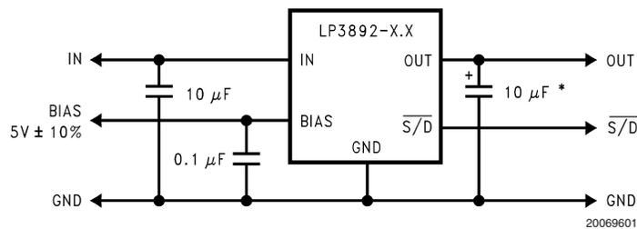
At least 10 µF of input and output capacitance is required for stability.
