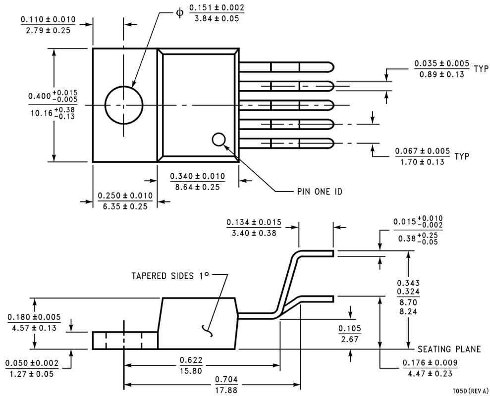
**TO220 5-lead, Molded, Stagger Bend Package (TO220-5)
