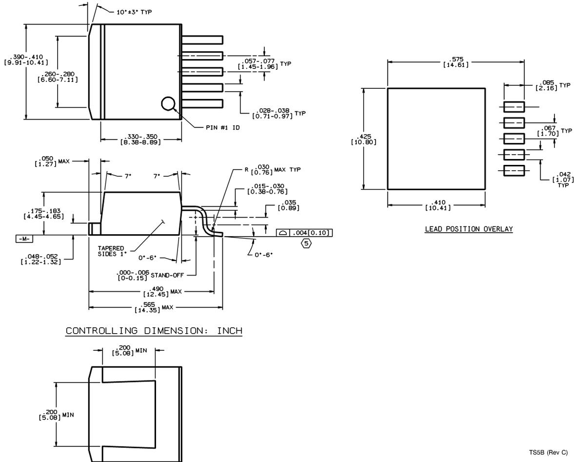
**TO263 5-Lead, Molded, Surface Mount Package (TO263-5)
